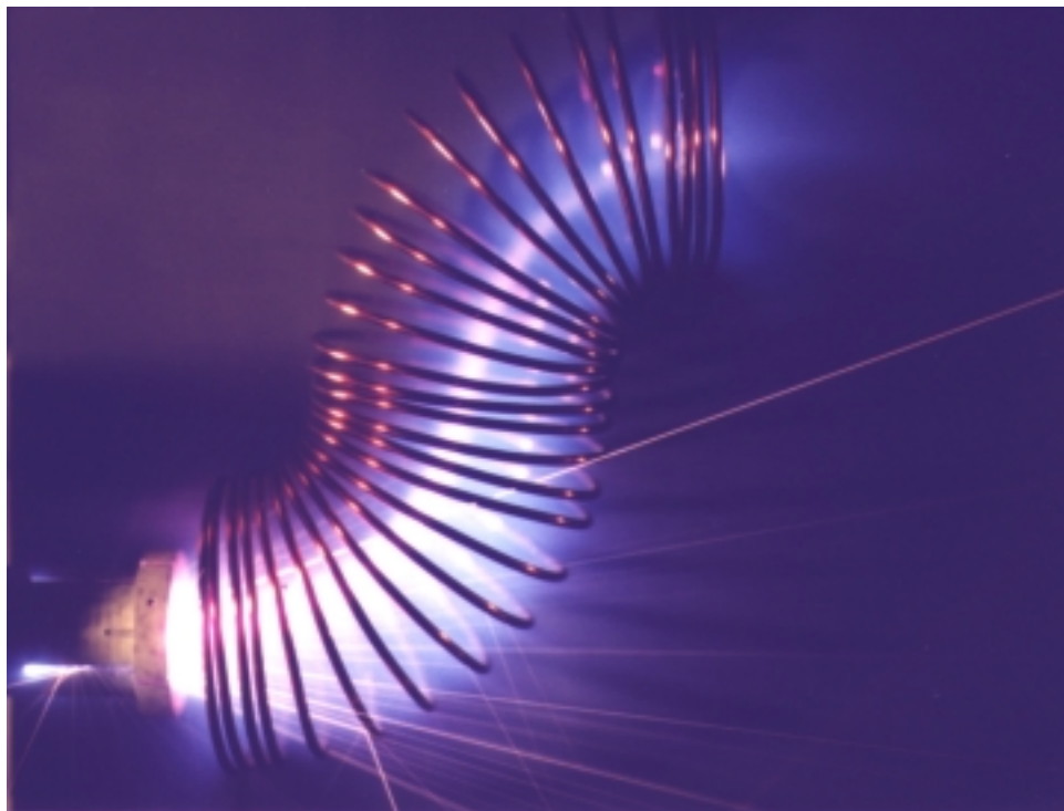
Figure 4. Open-walled S-duct filter in operation [33].
