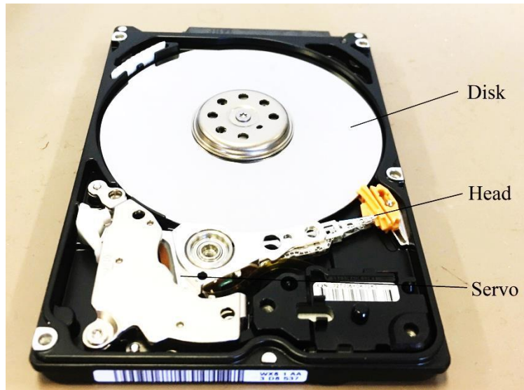
Fig. 1.1.1 Structure of a current commercial hard disk drive
