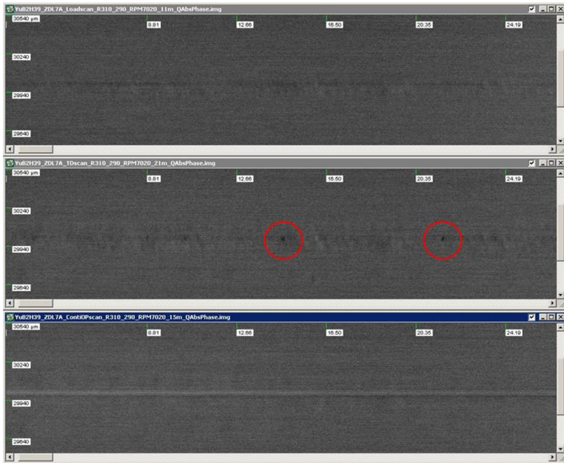
Figure. 5.5.1 Raw OSA image showing touchdown induced mogul formation (middle) on a Z-Dol 9 Å sample. (top) Topography of passive flying at 11 minutes, (middle) approximately 30 touchdowns and (bottom) continuous contacts in 900 seconds. Touchdown-induced moguls are circled in red.
