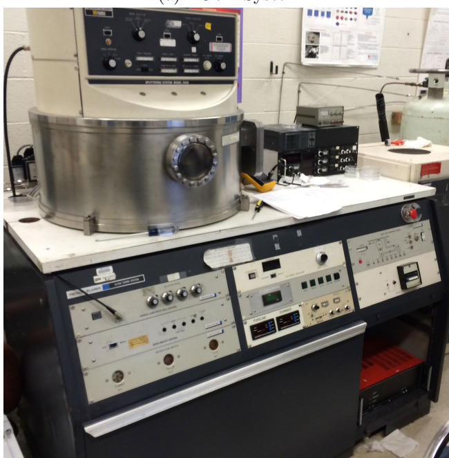
(b) RF Sputtering System (Perkine-Elmer Randex-2400 model)
