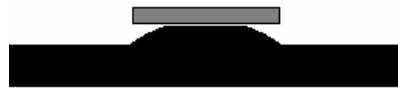
(a) A flat rigid slider in contact with a spherical asperity on the disk surface
