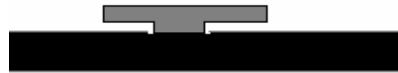
(b) A rigid slider with a flat pad in contact with a smooth disk
