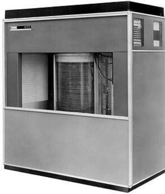
Figure 1.2: The IBM 350 Disk Storage System
