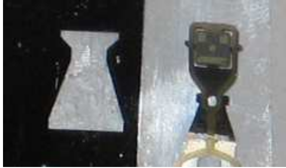
Figure 4.3. Completed wire bonding fixture (left)
