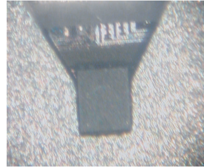
Figure 5.3. Slider located and mounted on microactuator using silicon fixture
