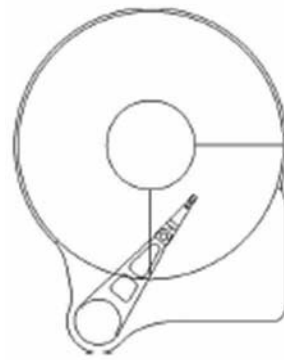
Figure 6.1: Generic hard disk drive model used for air flow simulations (C1) (From Kirpekar et al. [48])
