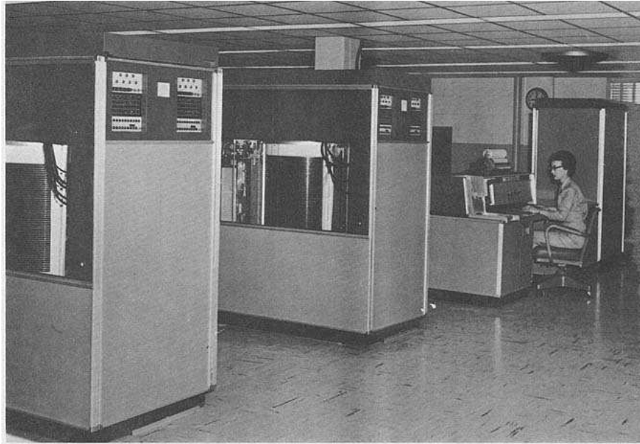
Figure 1.1. IBM 305 at U. S. Army Red River Arsenal Foreground: Two 350 disk drives. from Wikipedia (2006)
