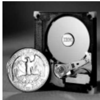
Figure 2.1: A typical rotary servomechanism of modern hard disk drives.
