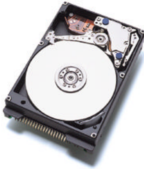
Fig. 1.1 The IBM Travelstar 25GB hard disk drive.
