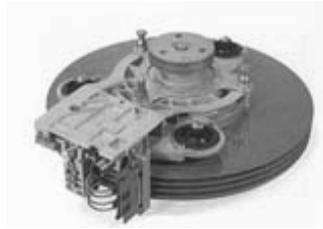
Figure 1.7: IBM 3340 disk drive of 1973, known as the "Winchester" drive.
