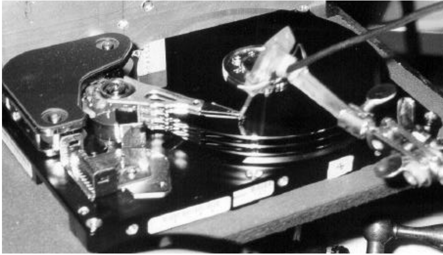
Fig. 1. Set up for flow measurement by hot wire.
