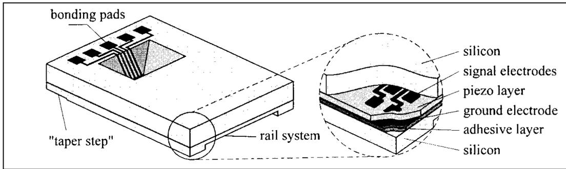
a) The silicon slider with sensor array
