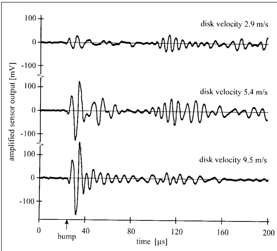
b) Typical sensor response on a interaction between the slider and the bump
