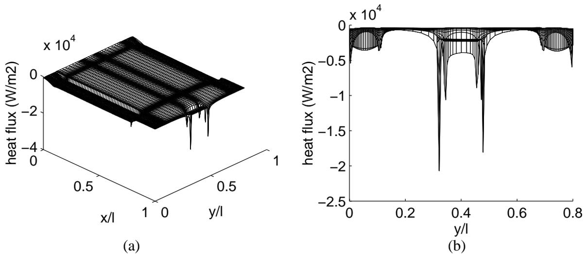
Fig.6 Heat flux between slider and the air bearing ( $T_s=T_d$ )
