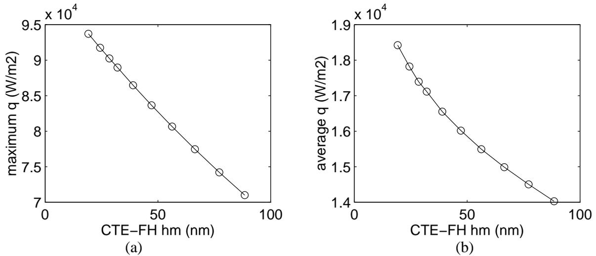
Fig.7 Heat flux vs. central trailing edge flying height ( $\Delta T = 1 \text{ }^\circ\text{K}$ )
