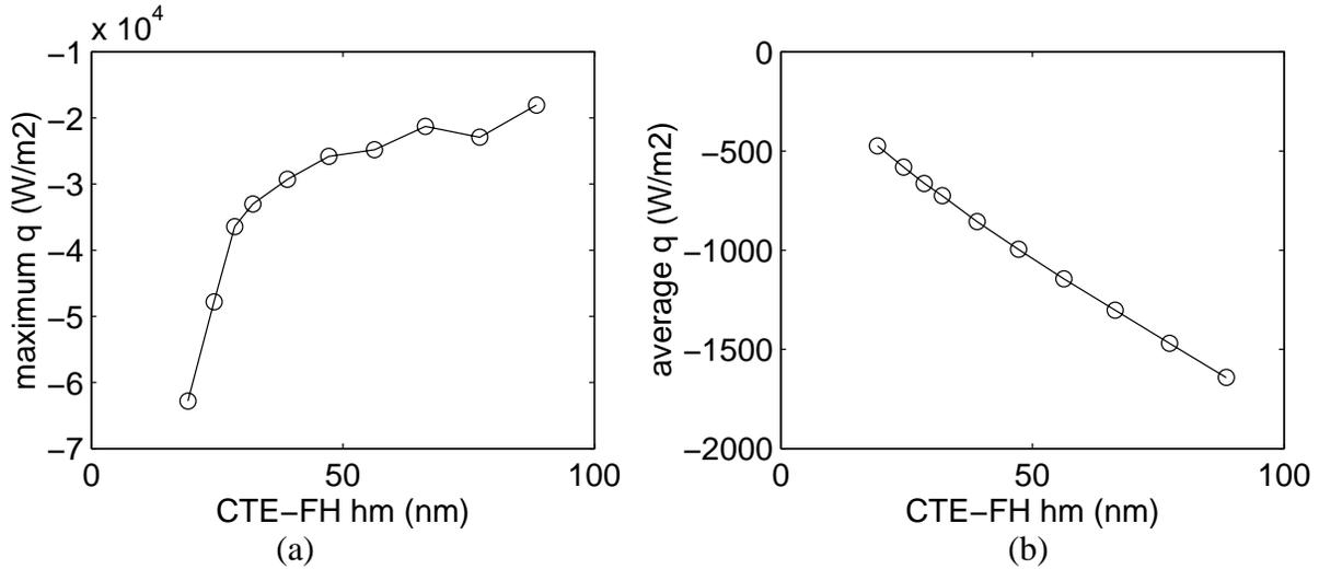
Fig.8 Heat flux vs. central trailing edge flying height ( $\Delta T=0 \text{ }^\circ K$ )
