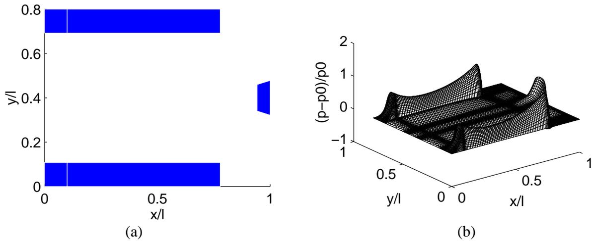
Fig. 4 A tri-pad slider and the pressure profile in the air bearing
