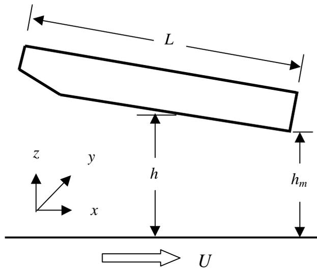
Fig.1 Slider/disk system and coordinates
