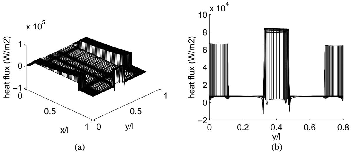
Fig.5 Heat flux between the slider and air bearing ( $T_s-T_d=1\text{ }^\circ K$ )
