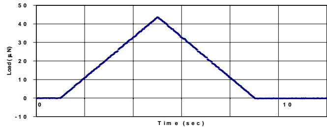
Figure 2 Load-Time Profile of nano-indentation using Hysitron Tester.
