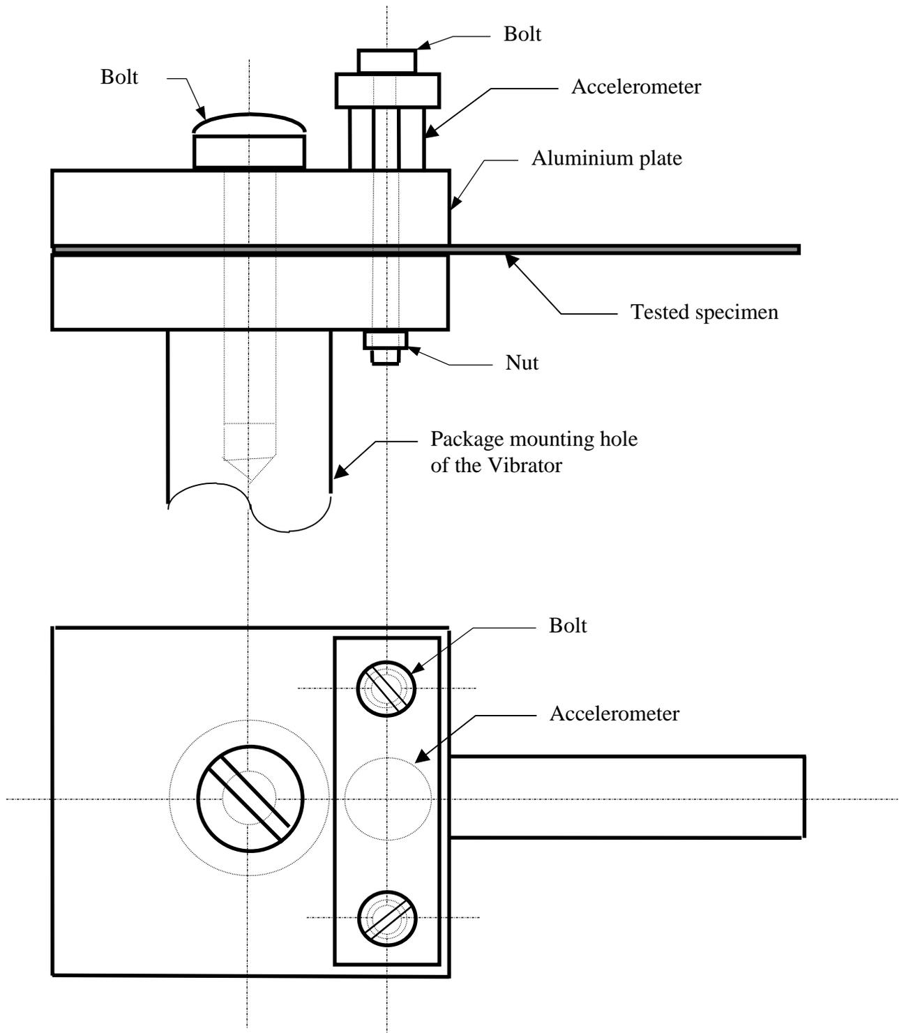
Figure 2 A fixture for the base excitation
