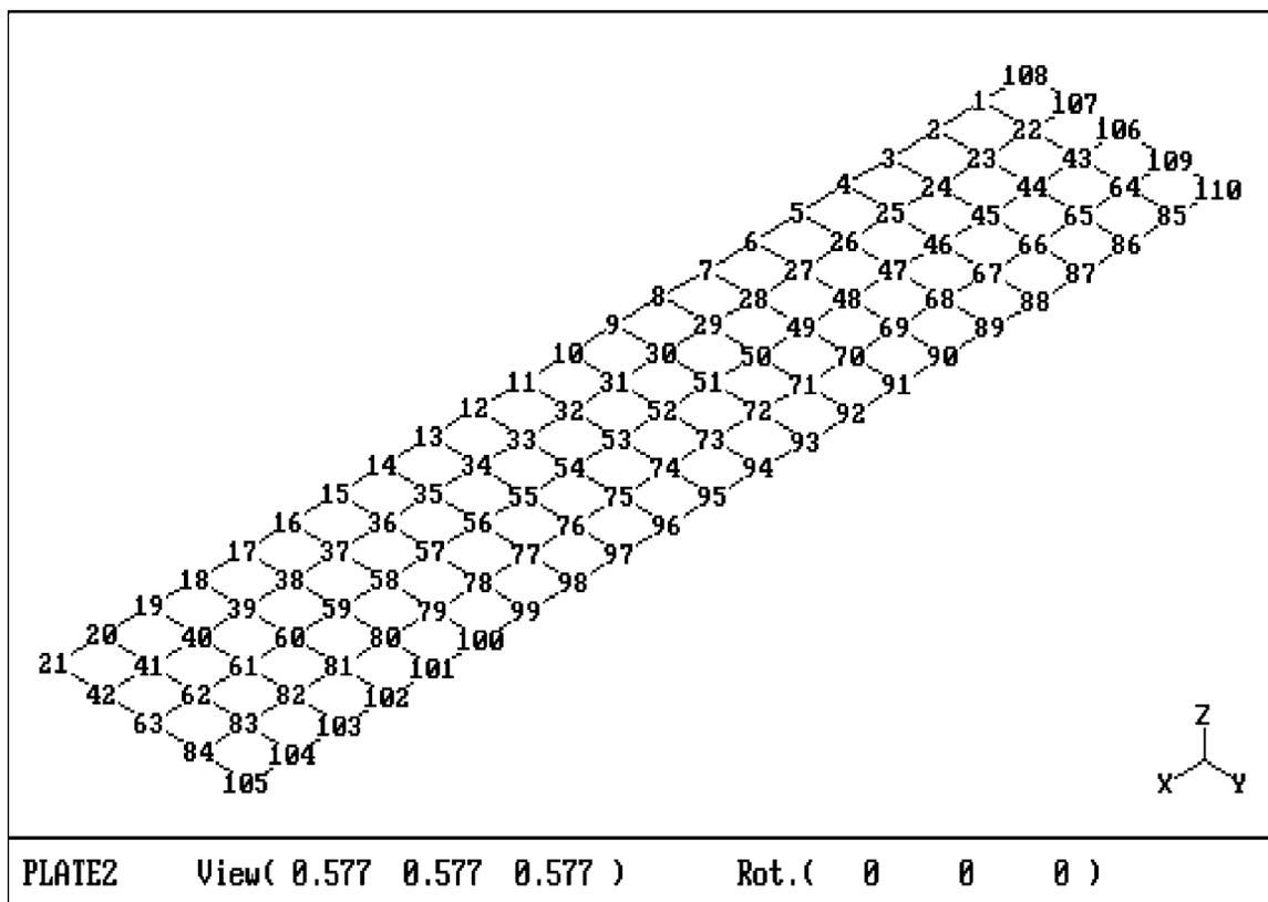
Figure 4 Geometric model of the cantilever plate
