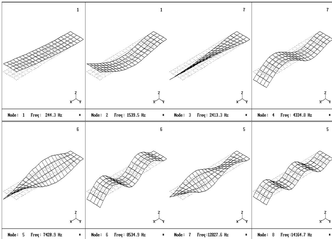
Figure 6 Measured mode shapes of the cantilever plate
