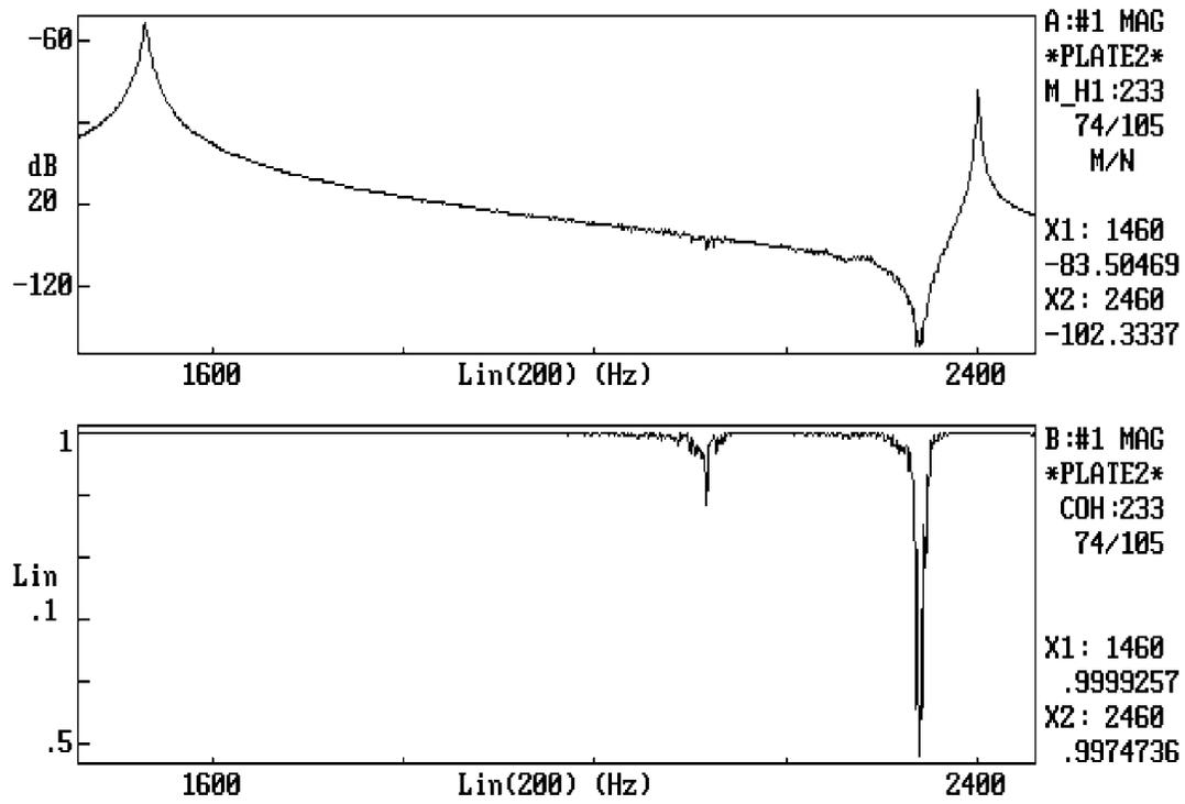
Figure 5 Measured FRF (upper) and coherence function (lower) of the plate at point 74
