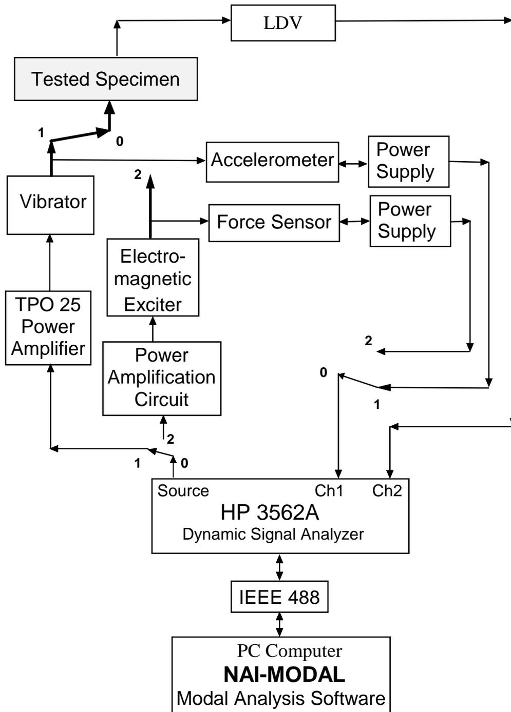
Figure 1 Schematic of the experimental modal analysis system
