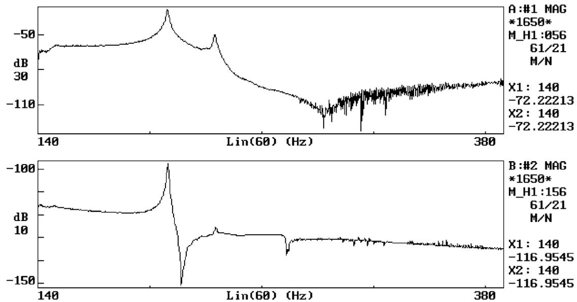
Figure 3 FRF calibration for the base excitation. The upper is the measured FRF, the lower is the calibrated FRF of the upper
