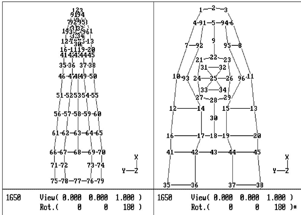
Figure 7 Geometric model of the type 1650 suspension
