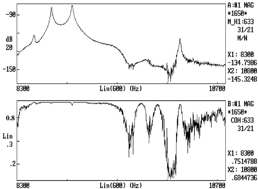
Figure 8 Measured FRF (upper) and coherence function (lower) of the type 1650 suspension at point 31
