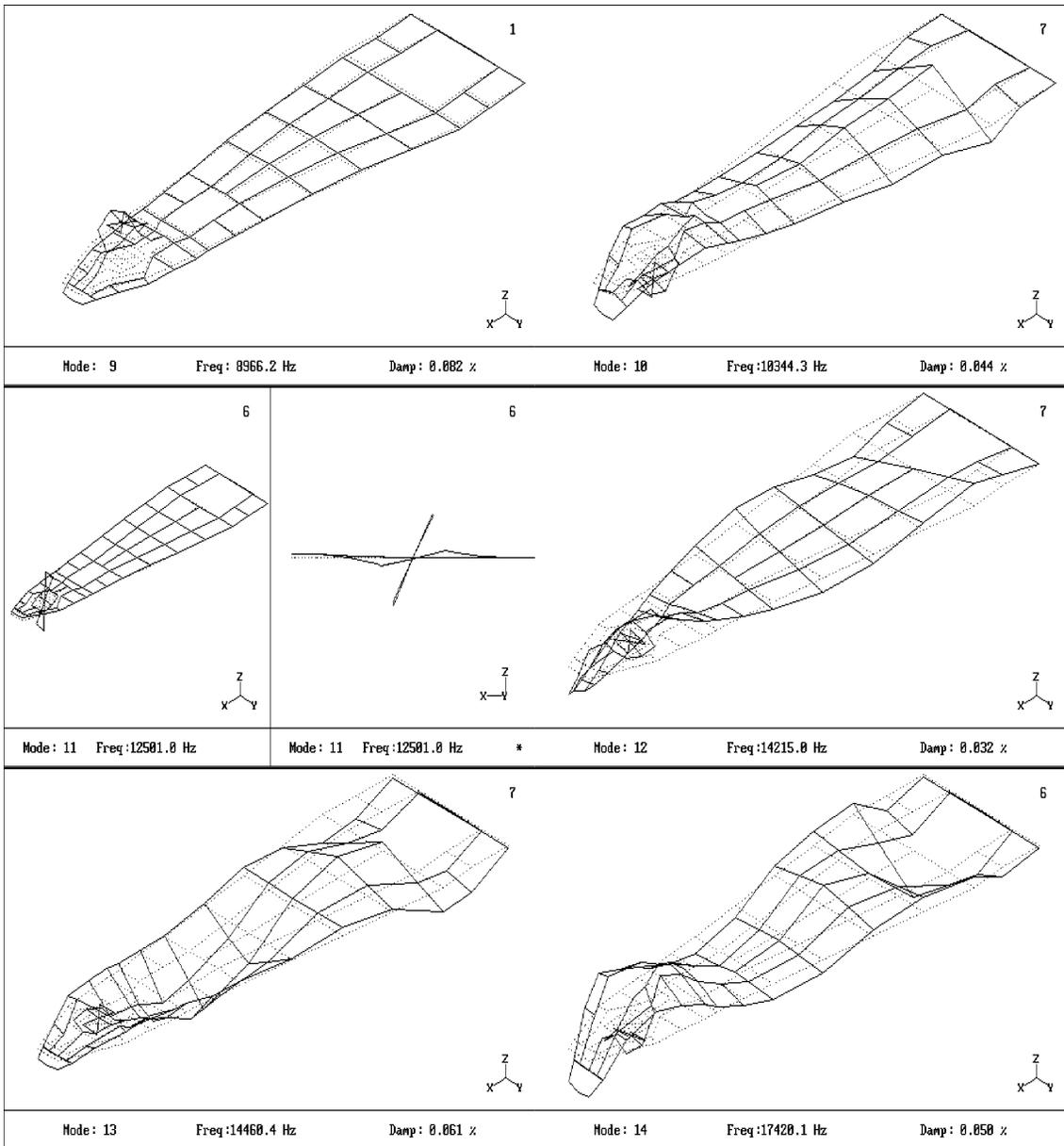
Figure 9 (continue) Measured mode shapes of the Type 1650 suspension
