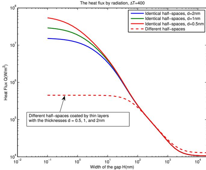
Figure 4: Radiative heat flux between coated and uncoated half-spaces at different temperatures
