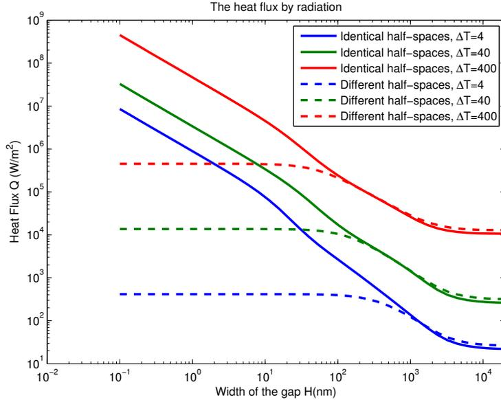
Figure 3: Radiative heat flux between two half-spaces at different temperatures
