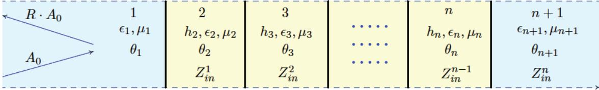
Figure 2: Computation of the reflection coefficient of a stack of layers
