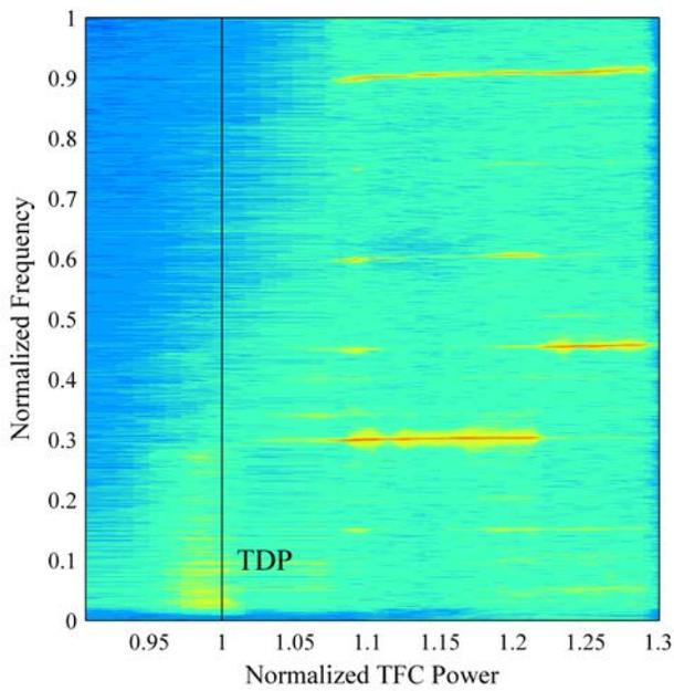
Fig. 6 Normalized TFC power-frequency spectrum contour of touchdown sensor signal
