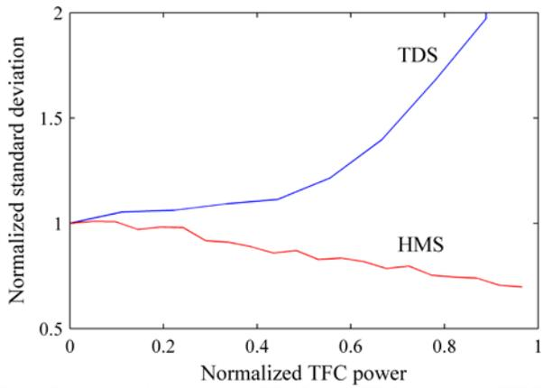
Fig.5 Standard deviation of HMS and TDS signal as TFC power increases during the passive flying stage
