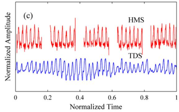
Fig. 4 HMS and TDS signal comparison at different stages: (a) passive flying stage, (b) transitional stage and (c) modulation stage.
