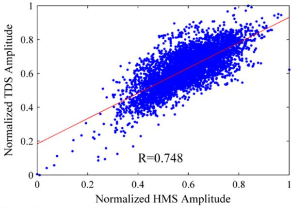
Fig.3 HMS and TDS signal correlation at the best phase shift
