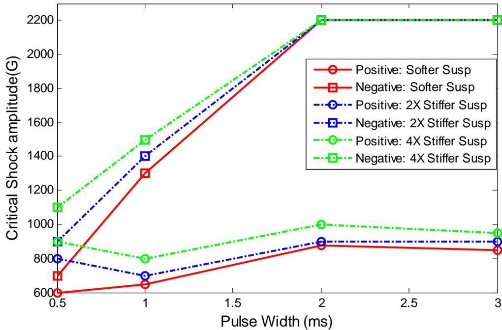
Figure 8 Critical shock dependence on pulse width for three flexure designs
