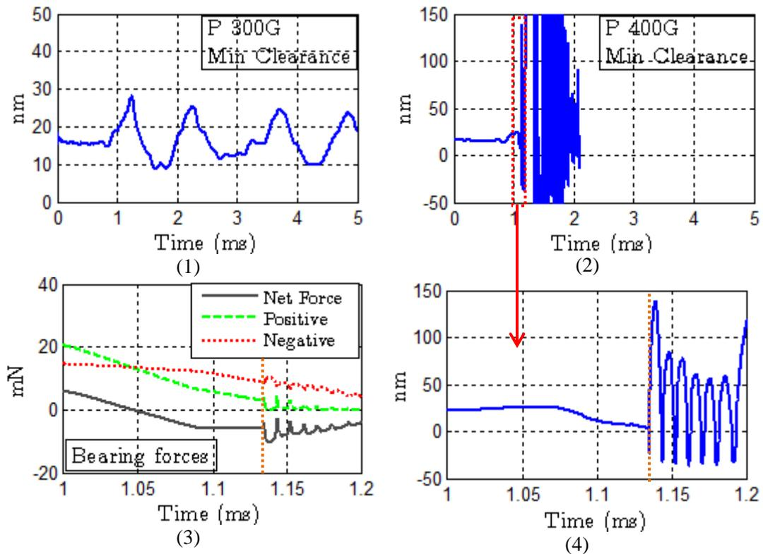
Figure 3 Failure mechanism for shock with short pulse width of 0.5 ms: (1) minimum clearance for positive shock 300 G - no failure; (2) minimum clearance for positive shock 400 G - failure; (3) air bearing force corresponding to the case in (2); (4) zoom in of minimum clearance in (2).
