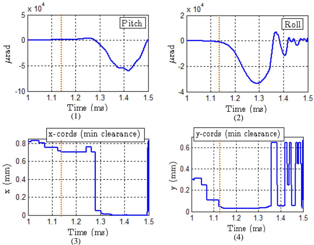
Figure 4 Slider's flying parameters for positive shock 400 G: (1) relative pitch; (2) relative roll; (3) x-coordinates for slider's minimum clearance point; (4) y-coordinates for slider's minimum clearance point.
