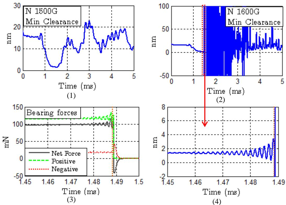
Figure 5 Failure mechanism for shock with long pulse width of 2.0 ms: (1) minimum clearance for negative shock 1500 G – no failure; (2) minimum clearance for negative shock 1600 G - failure; (3) air bearing force corresponding to the case in (2); (4) zoom in of minimum clearance in (2).
