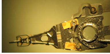
Figure 3: Picture of the Vector model PZT-actuated suspension used in our experimental setup
