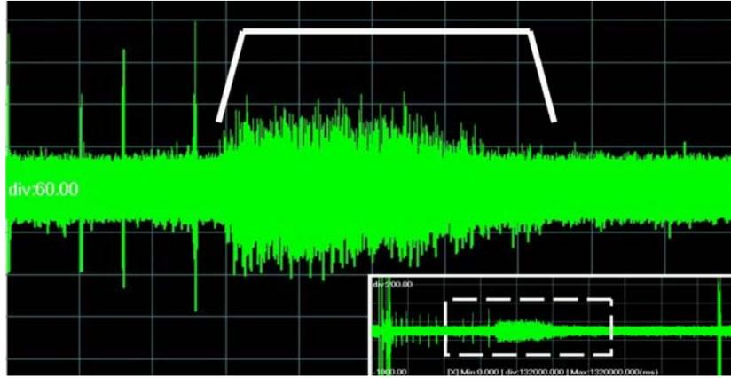
**Fig. 8.** LDV sensor data from lubricant dragging result, zoomed view of 4 to 14 minutes with broadened region bracketed. Inset shows the entire 20 minute test data with the 4 to 14 minute region outlined.
