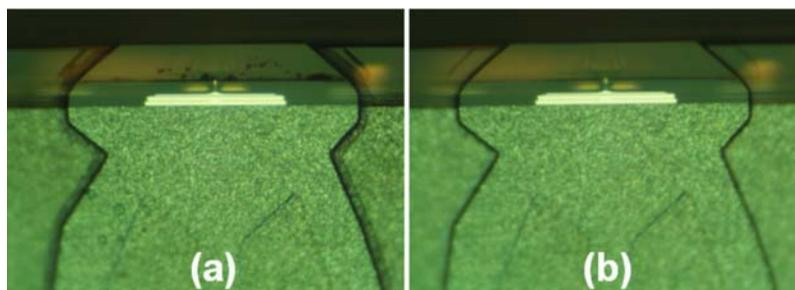
Fig. 7. Lubricant pickup at TEC (a) after a 20 minute on-track flying test (b) after cleaning with HFE ultrasonic bath.
