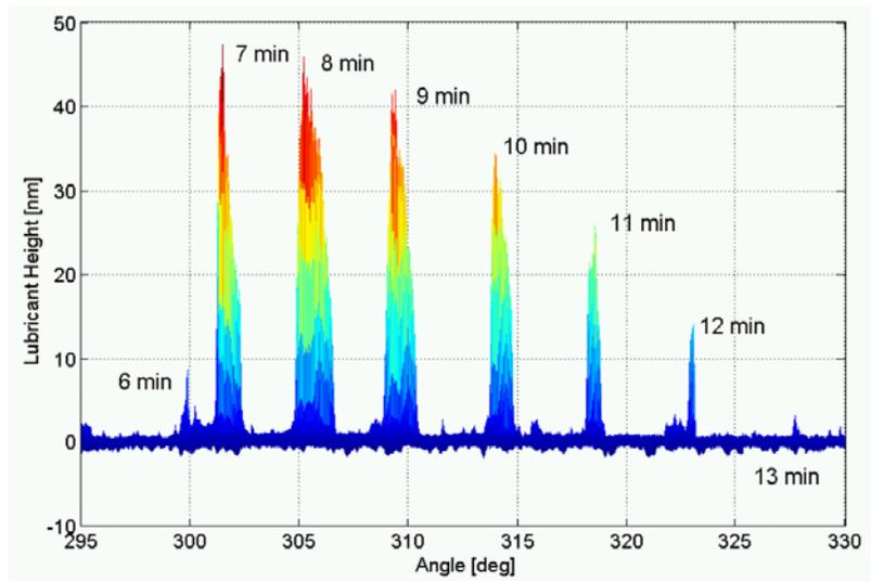
**Fig. 10. Angular view of lubricant droplet height data as it moves down-track with successive OSA scans (6 min to 13 min).**
