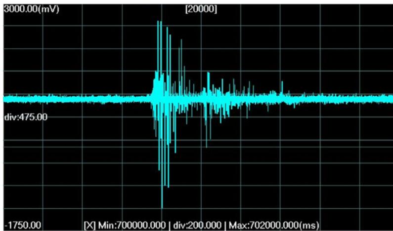
**Fig. 2. Example AE sensor spike (x-axis length is 2 seconds).**
