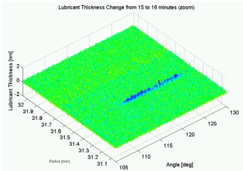
Fig. 5. Lubricant height from 16 minute – 15 minute data showing 1 mm x 25 degree area around lubricant drop (oblique view).
