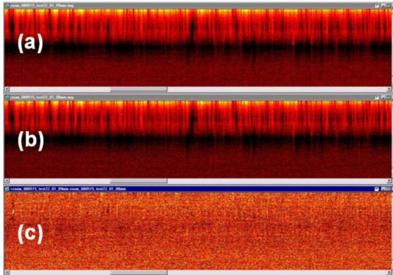
**Fig. 3.** OSA screenshot showing lubricant thickness over 500  $\mu\text{m}$  x 54 degree area (darker = thicker) showing an interval with no lubricant droplets or AE/LDV spikes (a) 9 minute – base (b) 8 minute – base (c) 9 minute – 8 minute.
