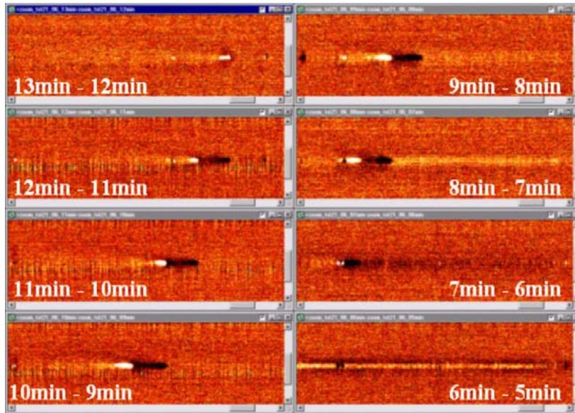
**Fig. 9.** OSA screenshot of changes in lubricant thickness between scans over 350  $\mu\text{m}$  x 27 degree area (darker = thicker) showing down-track motion of a large lubricant droplet (down-track is to the right of each frame).
