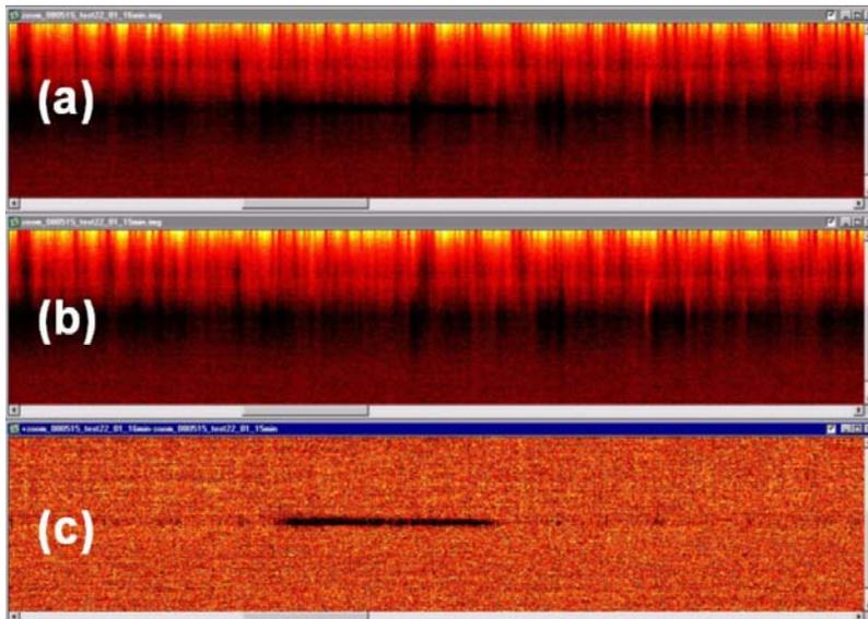
**Fig. 4.** OSA screenshot showing lubricant thickness over 500  $\mu\text{m}$  x 54 degree area (darker = thicker) showing a lubricant droplet (a) 15 minute – base (b) 16 minute – base (c) 16 minute – 15 minute.
