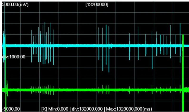
**Fig. 1. AE (top) and LDV (bottom) data showing intermittent spikes during a 20-minute flying test at approximately 30m/s linear speed.**
