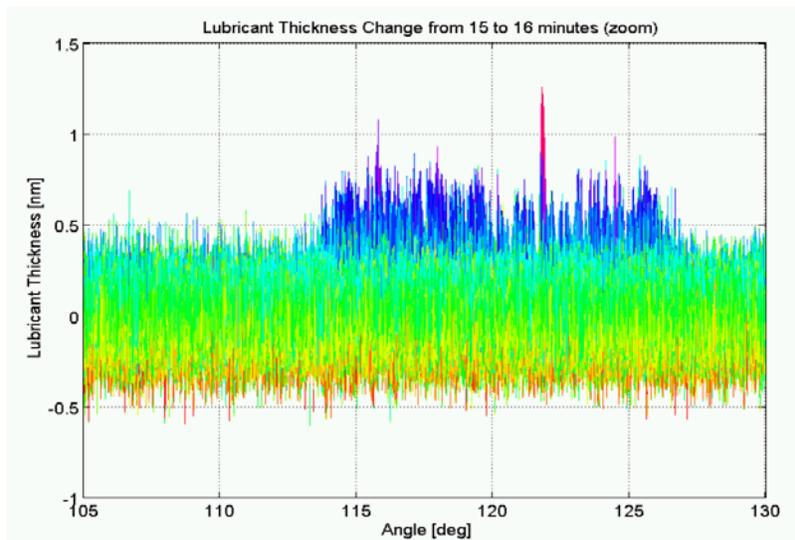
Fig. 6. Lubricant height from 16 minute – 15 minute data showing 1 mm x 25 degree area around lubricant drop (angular view).
