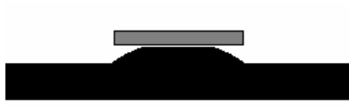
(a) A flat rigid slider in contact with a spherical asperity on the disk surface
