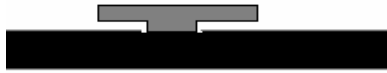
(b) A rigid slider with a flat pad in contact with a smooth disk
