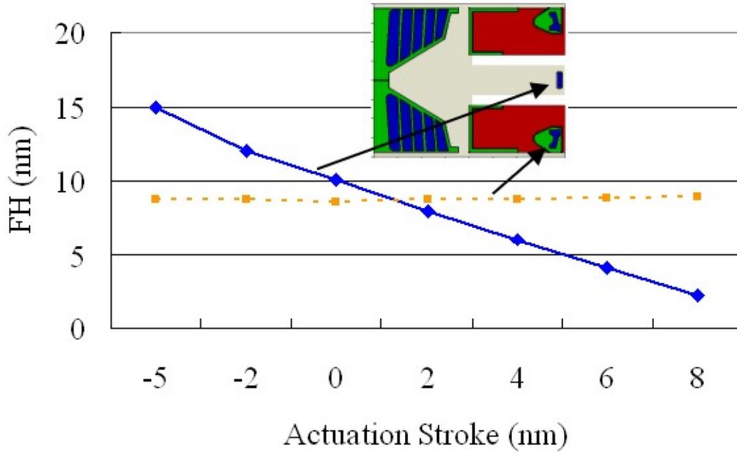
Fig. 6. Simulated FHs at the read/write transducer and one point on one of the side ABS rails. The radial position is at the MD.
