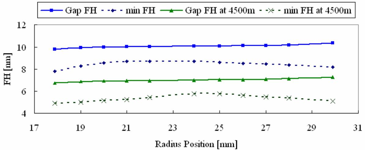
Fig. 4. Simulation of gap FH and minimum FH profiles of Scorpion IV at sea level, 0 m, and high altitude, 4500 m.
