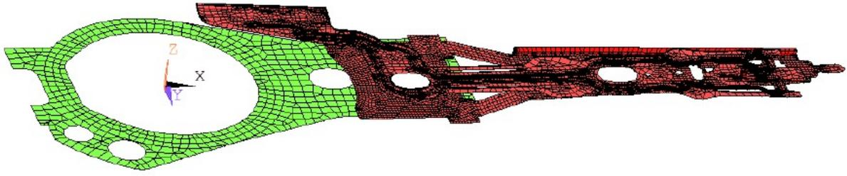
Fig. 14. Suspension model used in the dynamic load/unload simulation [27].
