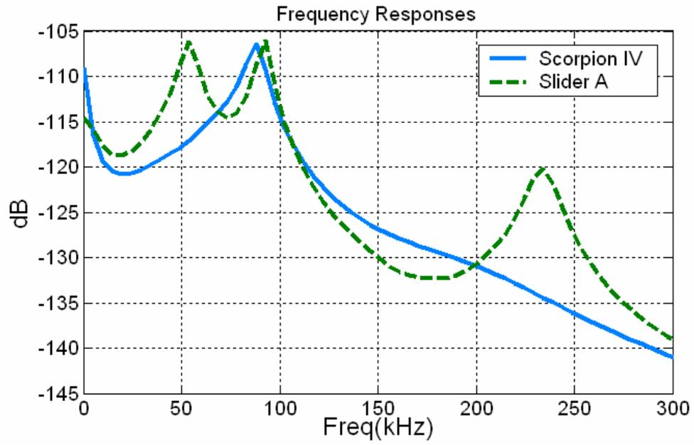
Fig. 8. Frequency responses of the air bearings of Scorpion IV and Slider A.
