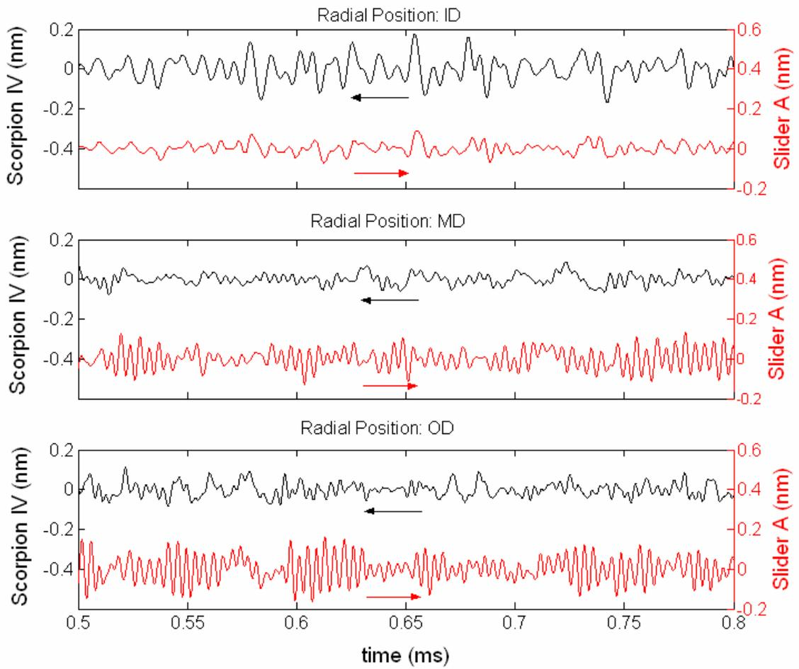
Fig. 20. Comparison of FHMs of Scorpion IV and Slider A at three radial positions, ID, MD, and OD with skews  $-15.62^\circ$ ,  $-2.56^\circ$ , and  $7.22^\circ$ , respectively.
