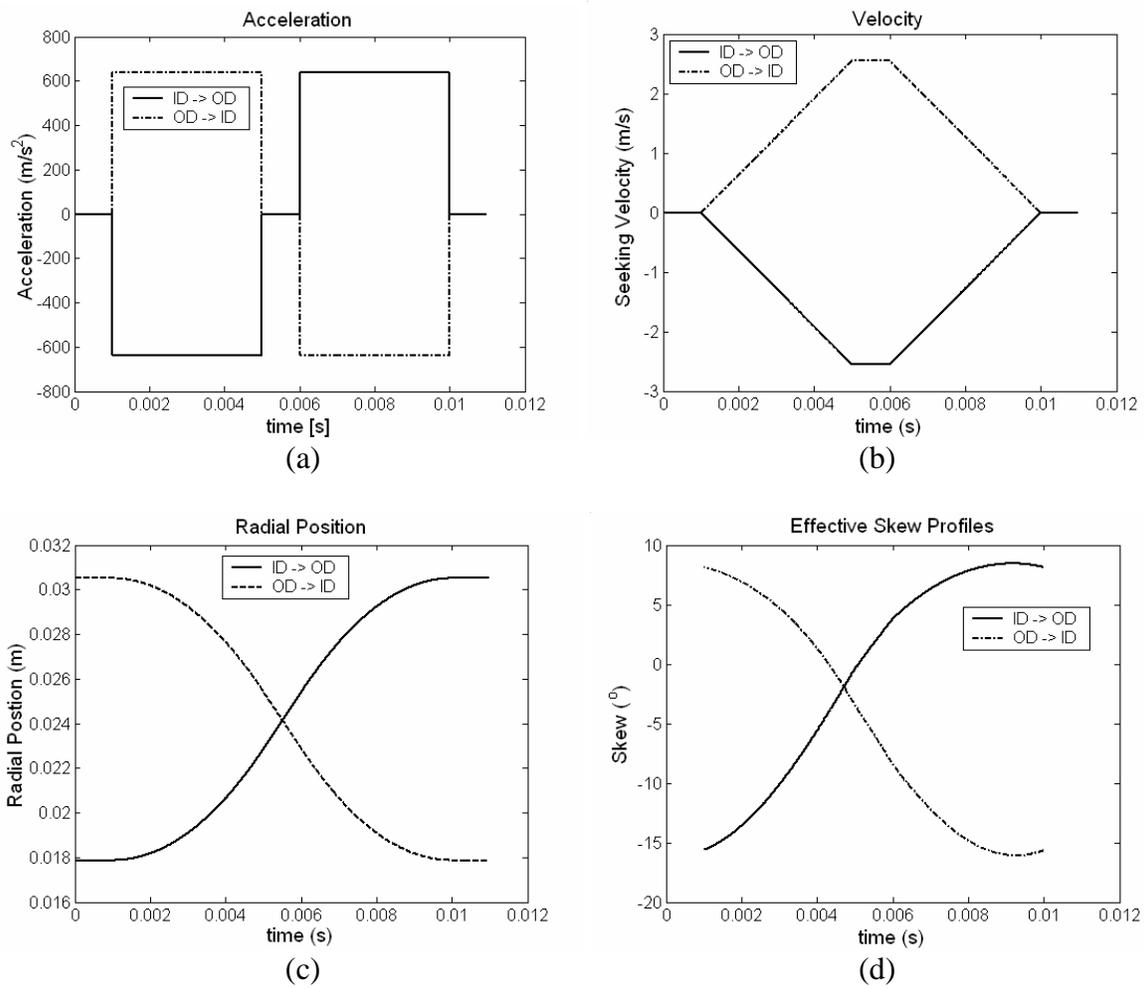
Fig. 12. Track-seeking profiles. The maximum acceleration is 65 G.
