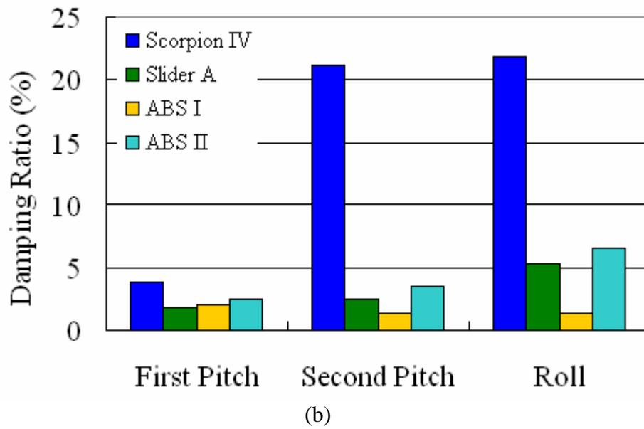
Fig. 9. Comparison of modal frequencies and damping ratios of various ABS designs. The data of Scorpion IV and Slider A were evaluated at the MD. The data of ABS I and ABS II were obtained from [24].
