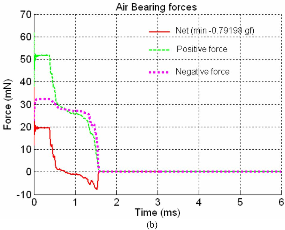
Fig. 17. Air bearing force histories during unloading processes at the OD. (a) unloading velocity: 50 mm/s; (b) 150 mm/s.
