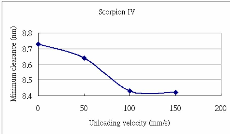
Fig. 16. The minimum clearances during the unloading process as a function of unloading velocity.
