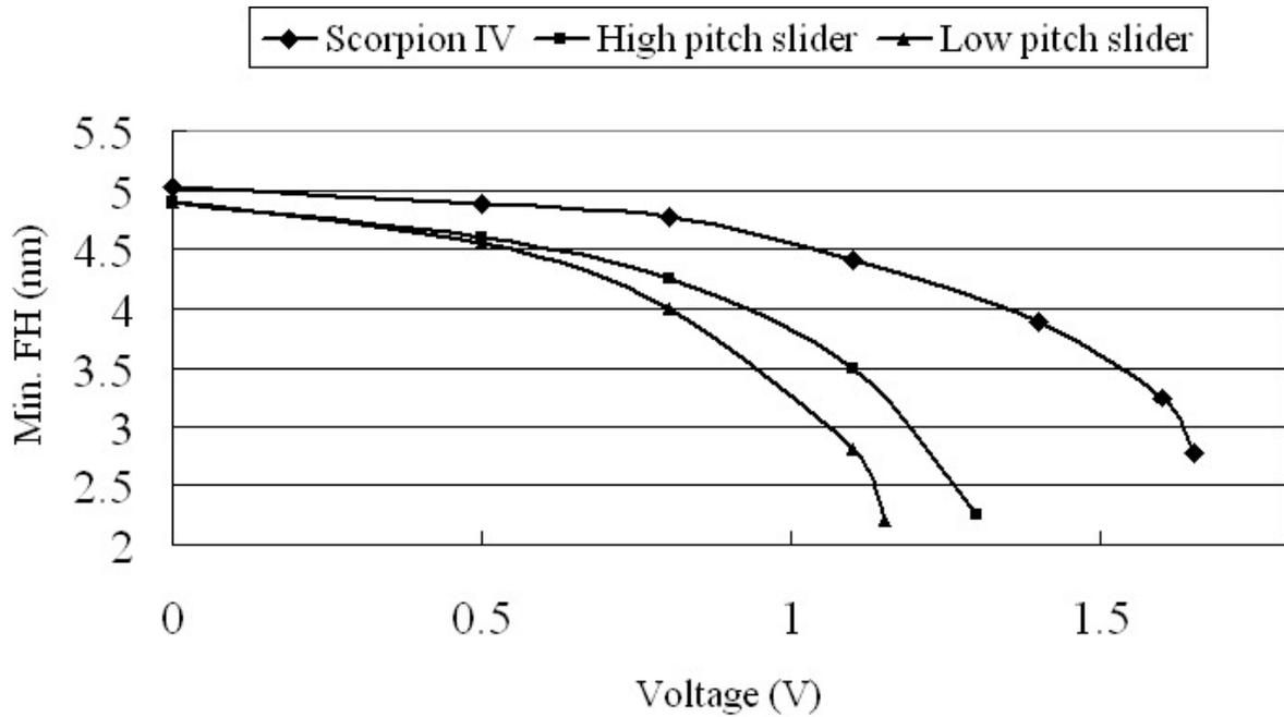
Fig. 10. The drop of minimum FH caused by the electrostatic potential across the HDI. The actuation stroke of Scorpion IV is 4 nm. The pitch of Scorpion IV is 108  $\mu$ rad at zero voltage. The results of the high-pitch slider (245  $\mu$ rad) and low-pitch slider (190  $\mu$ rad) are from [26].
