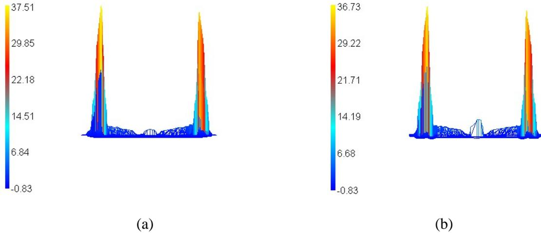
Fig. 7. Air pressure distributions before (a) and after (b) a 8-nm actuation stroke.
