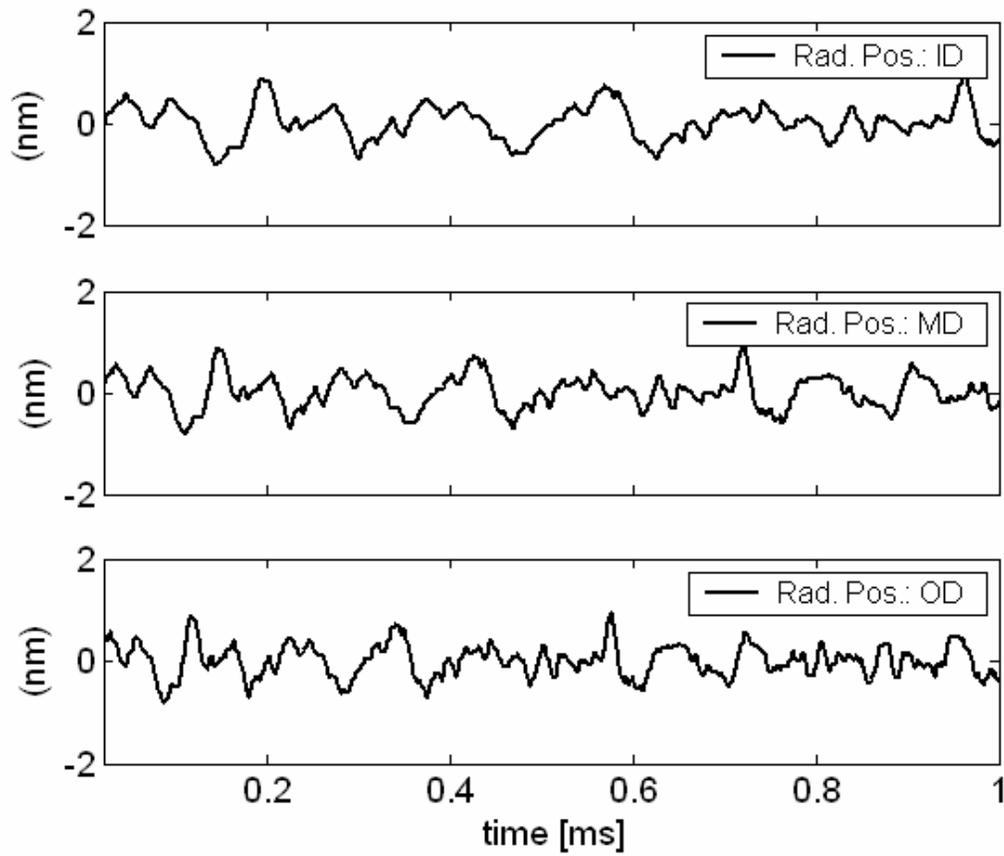
Fig. 19. Measured disk morphology used in the simulation at three radial positions, ID, MD, and OD. The peak-to-peak and standard deviation of the disk roughness are 1.76 nm and 0.31 nm, respectively.
