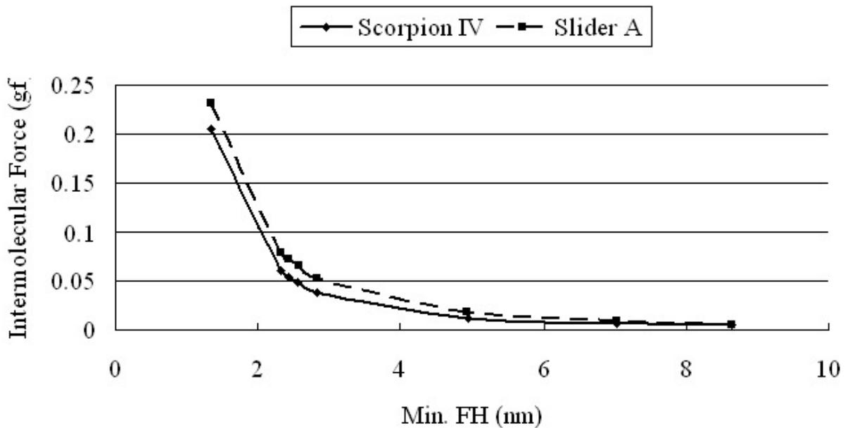
Fig. 11. Comparison of magnitudes of intermolecular adhesion forces of Scorpion IV and Slider A as a function of minimum FH. The FH of Scorpion IV was reduced by actuating the central trailing pad toward the disk and the obtained flying attitudes (min. FH, pitch, and roll) were then used to calculate the intermolecular forces of Slider A.
