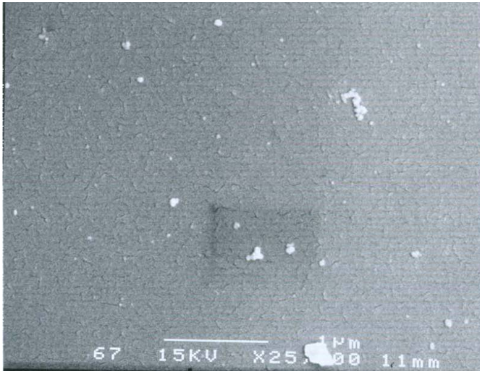
Fig. 9 Electropolished, x25,000, 10 min, ~ 3.5V, room temperature
