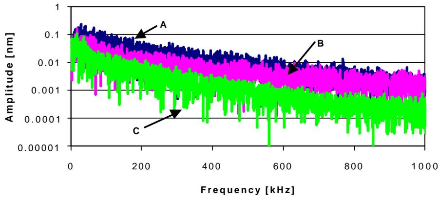
**Fig. 3: Power spectral density of disks A, B and C morphologies as seen from a stationary point as the disk rotates.**
