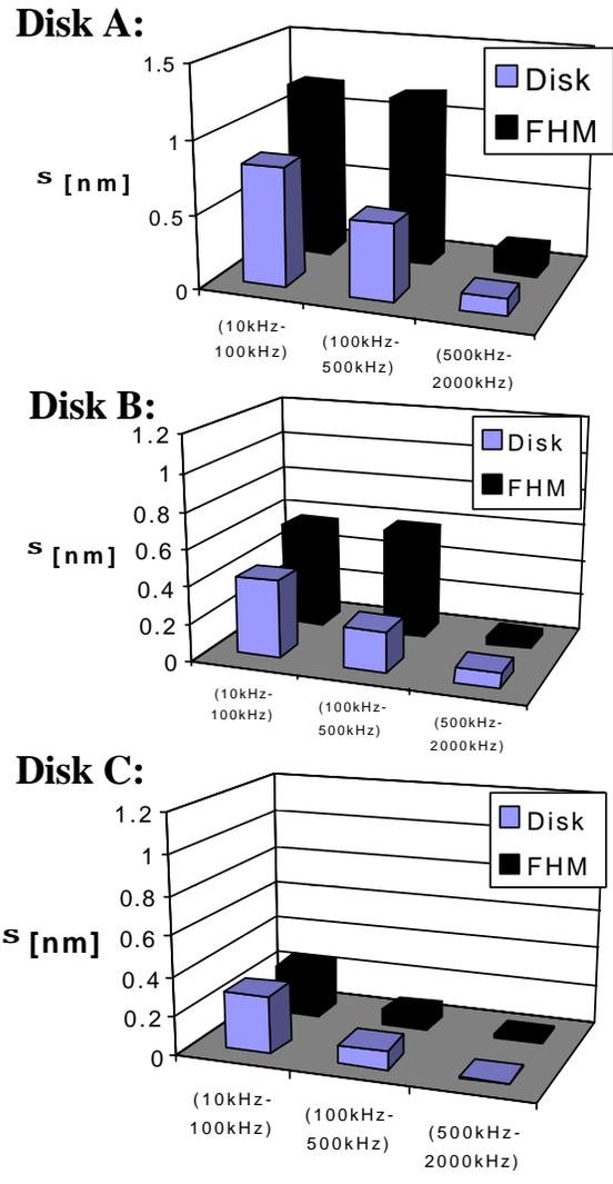
**Fig. 7: Standard deviation of disk morphologies and FHM for disks A, B and C broken into the three Bands; Band I: 10kHz-100kHz, Band II: 100kHz-500kHz and Band III: >500kHz.**
