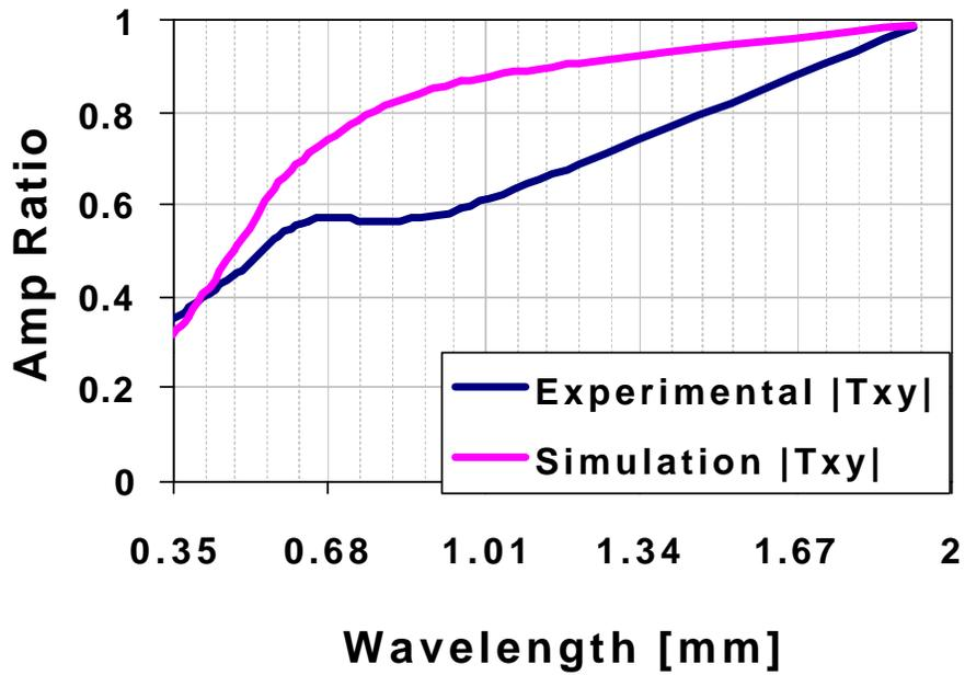
Fig. 9: Amplitude ratio of the slider to the disk displacement as a function of wavelength on the disk morphology.
