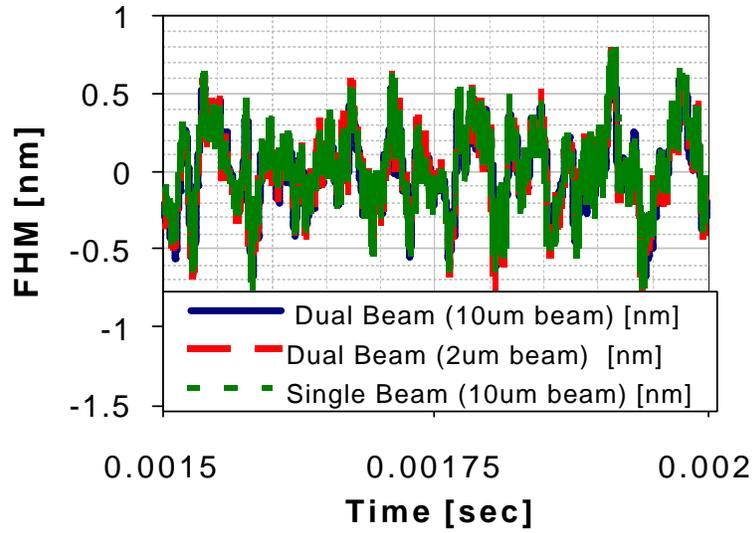
**Fig. 1: FHM comparison between dual beam and single beam LDV measurements.**
