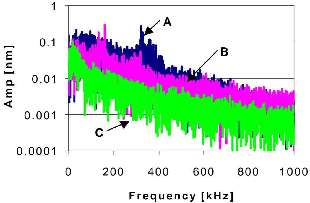
**Fig. 4: Power spectral density of the FHM at the transducer location for disks A, B, and C.**
