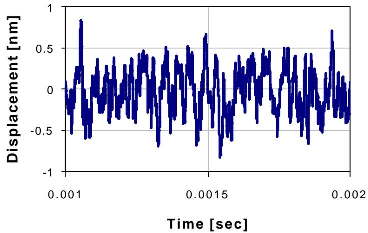
**Fig. 5: Measured disk morphology of disk C used in the simulation.**
