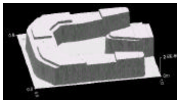
FIG. 23. The 3-D geometry of the NSIC slider.
